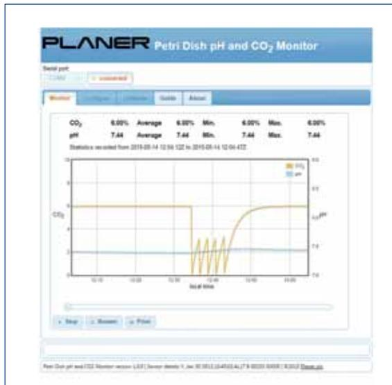
Figure 3. Monitoring of both the culture chamber CO<sub>2</sub> levels and corresponding predicted pH following multiple lid openings in a benchtop incubator.
