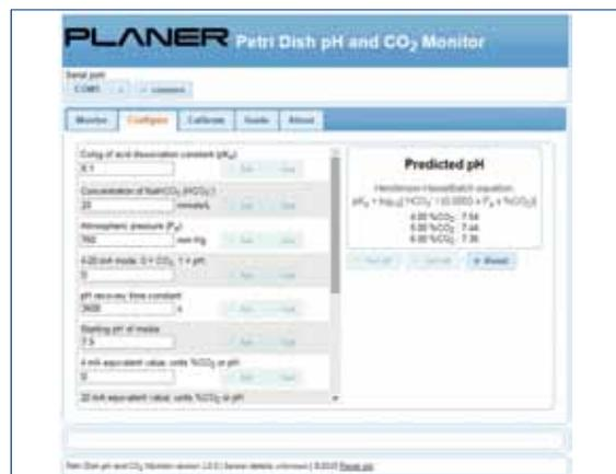
Figure 2. Configure tab of the Petri dish pH / CO<sub>2</sub> application allows input of parameters used to determine pH in an established culture system
