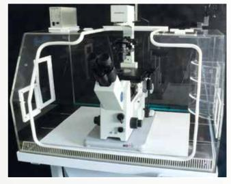
Fitting a microscope and ancillary equipment is easy via the large removable front section of the chamber.
