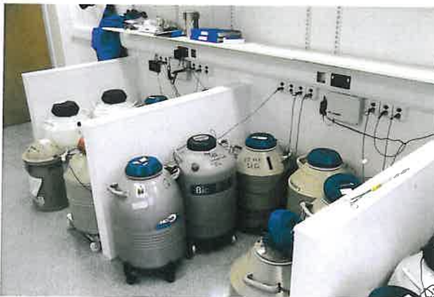
Storage Dewars set up for web-based monitoring.
