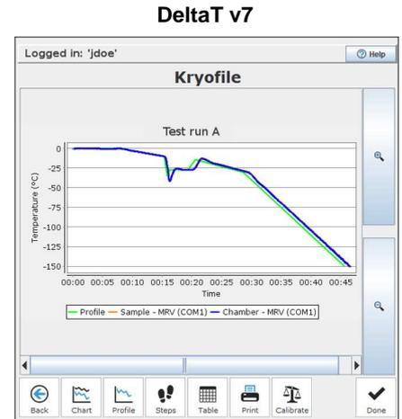
DeltaT provides a PC interface for the Planer range of controlled rate freezers allowing you to rapidly develop and maintain profiles on your PC and view freezing progress in real time.
